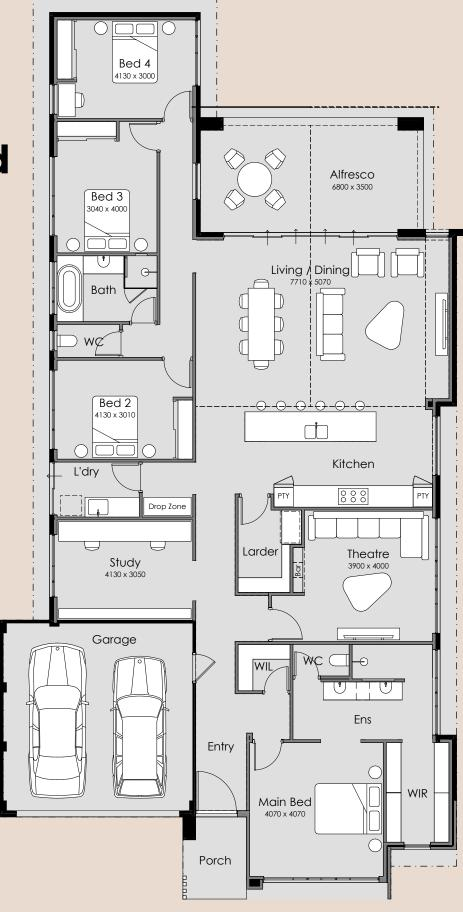
Overall Width – 13.89m Overall Length – 26.99m Min Block Width – 15.00m Min Block Length – 30.00m Total Area – 294.58m<sup>2</sup>
