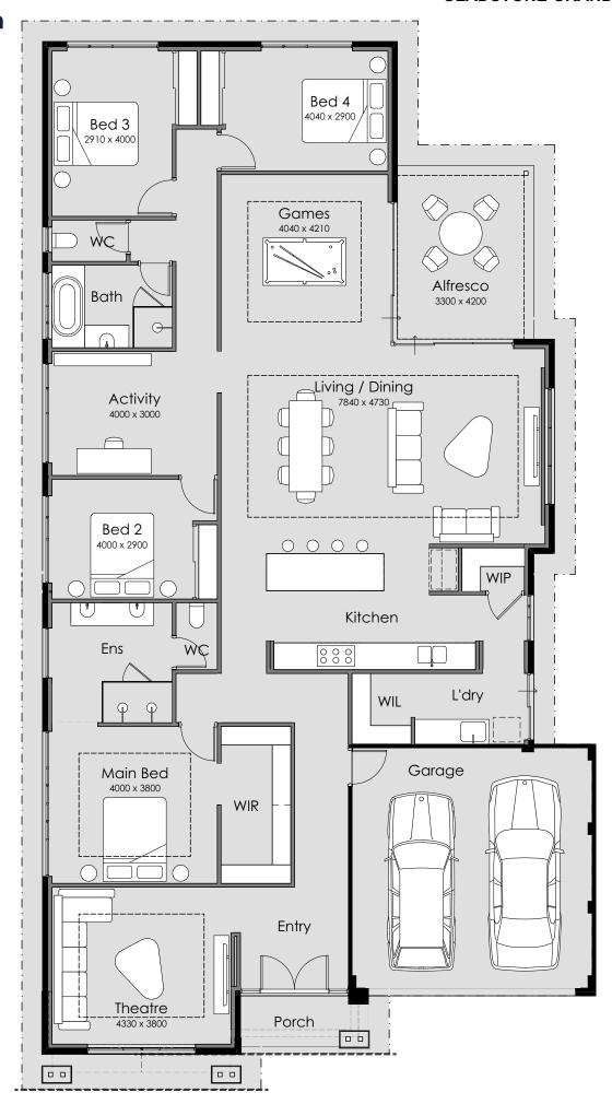
OVERALL WIDTH- 13.39m OVERALL LENGTH- 25.19m MIN BLOCK WIDTH- 15.00m MIN BLOCK LENGTH- 30.00m TOTAL AREA- 286.92m<sup>2</sup>
